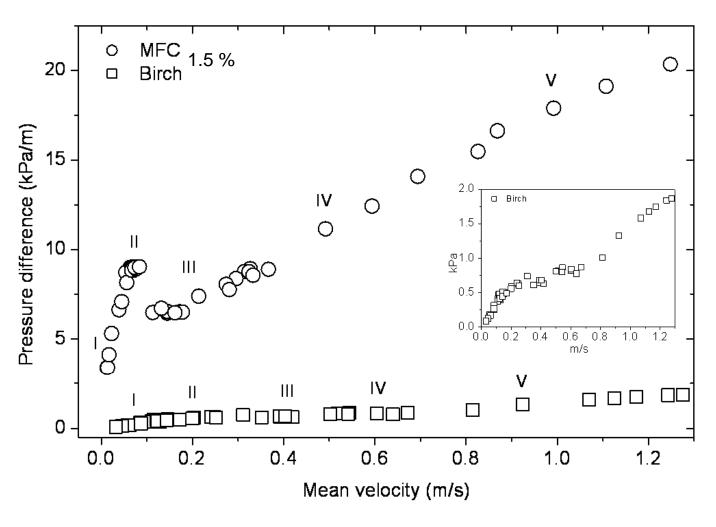
Similar flow regions than for normal fibre suspension flow was found for MFC
