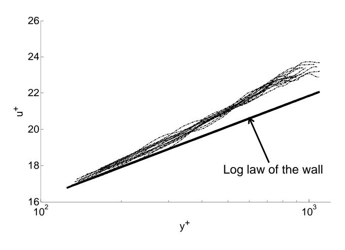
The measured velocity profile of a pure water matches closely with the theoretical log law of wall curve
